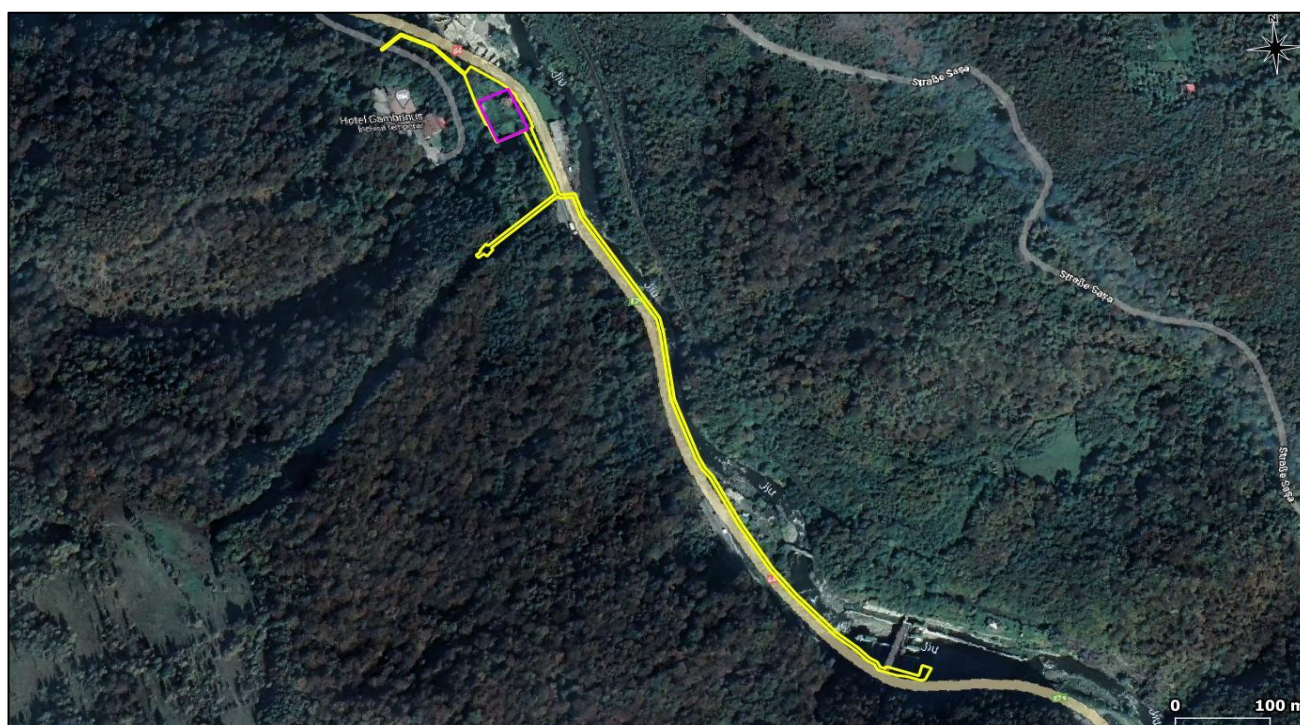
Fig. 49 Territorial framing of the areas concerned by the implementation of the project component aimed at connecting CHE Dumitra to the SEN (yellow polygons - power line routes, purple polygon - 110 kV transformer station)
