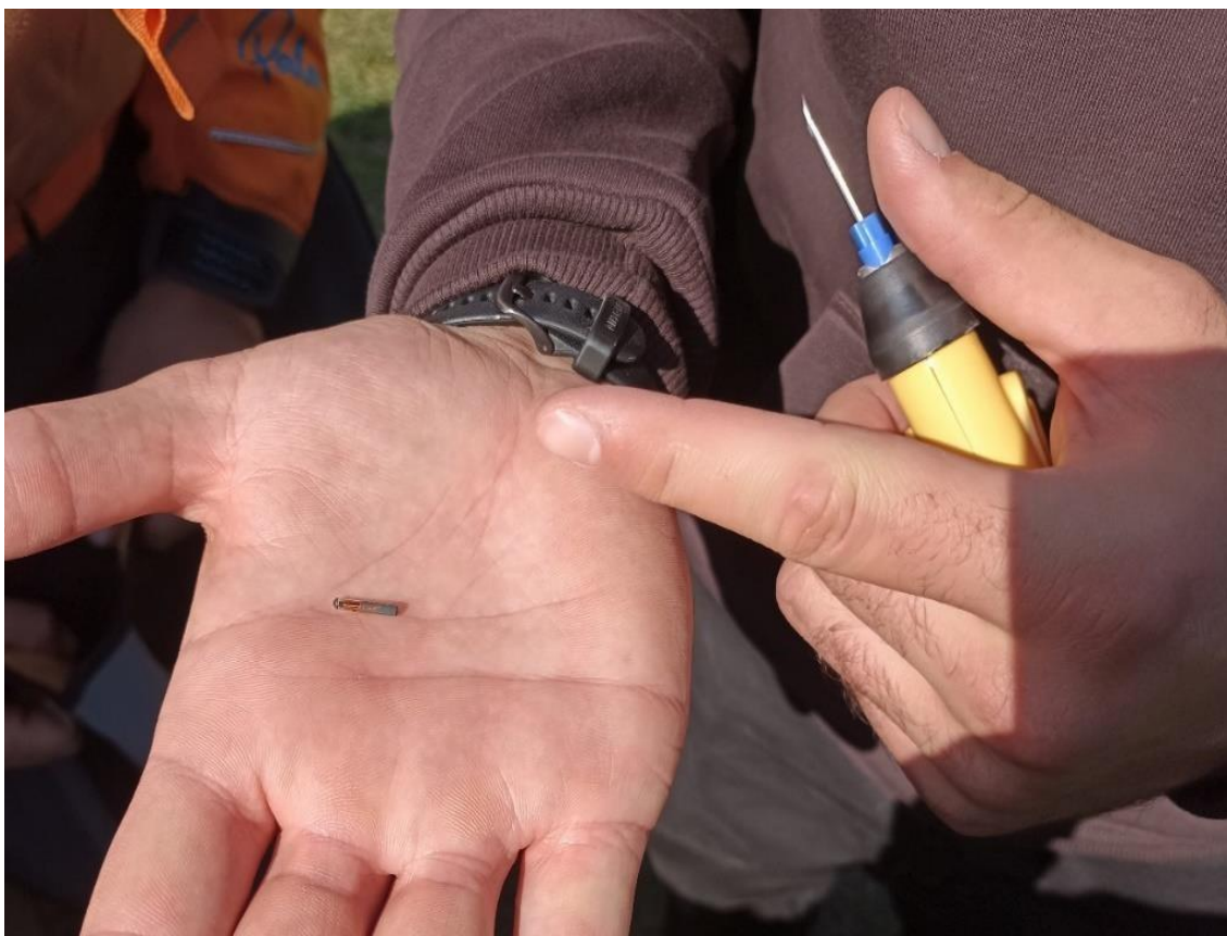
Fig. 182 Example of "PIT Tag" + needle and gun used for marking fish species for monitoring fish ladders.
